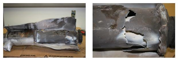
**Figure 2.** Fractured exhaust muffler from a Hefty Polar Cub airplane (left) and a close-up photograph of the fracture in the exhaust muffler (right).
