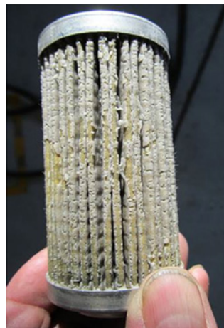
Figure 2. DEF crystals in fuel filter. PHOTO COURTESY OF FAA
