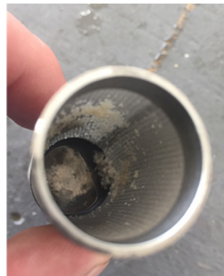
Figure 1. Fuel screen contaminated with DEF crystals following the 2019 fuel contamination event.
